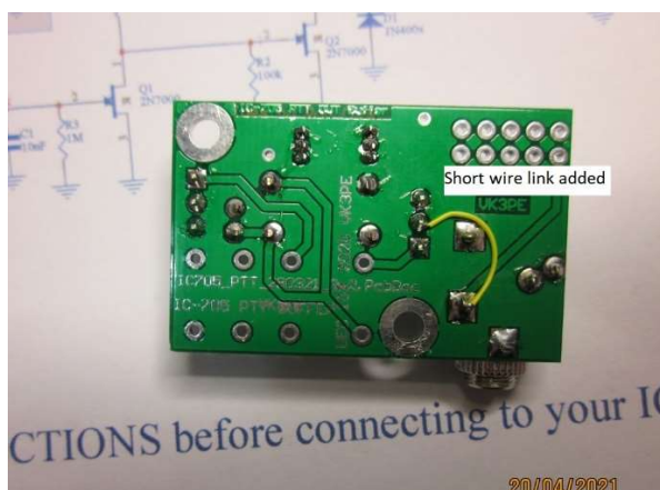
Wire link using some wire wrap wire in this case:
