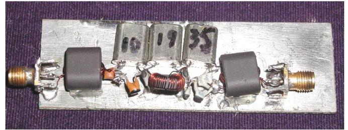
To achieve the desired bandwidth, which is relatively wide for a ladder crystal filter, balanced transformers with neutralization capacitors are used on the end sections and a neutralization inductor is used in the middle section.
